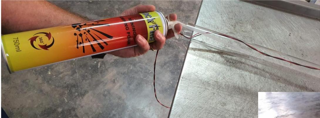
One can of 750 ml ROCK FILLA MINING TAMPING FOAM should under good conditions expand to make 35.5 liters of foam.
