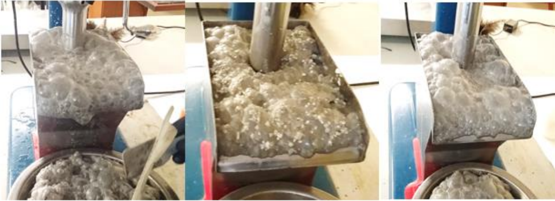
Figure 2 (from left to right) Normal flotation response. After Rock Filla addition. One minute into hot float with Rock Filla.
