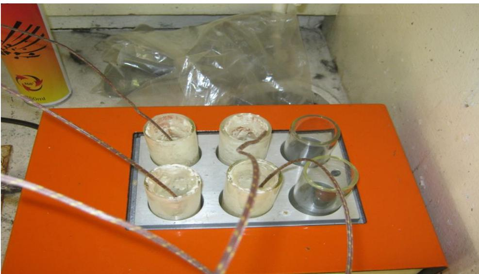
**Fig 3.** Test tubes containing foam and emulsion with thermocouples placed in the heater block
